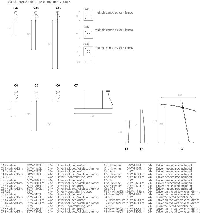
D. on the wire/Controller incl. Driver on the wire/wireless dimm. Driver on the wire/wireless dimm. D. on the wire/Contr. incl.
